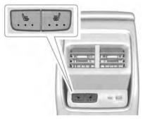
If equipped, the rear heated seat buttons are on the rear of the centre console.
