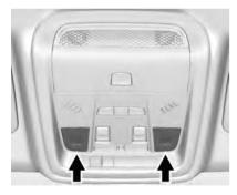
Press the lamp lenses to turn the front reading lamps on or off.
