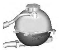
If topping up the level in the coolant surge tank, add the proper mixture until the level reaches the mark on the front of the tank and replace the cap. Operate the vehicle. Repeat steps 1–3, as necessary.
