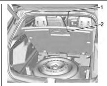
Insert the hook (2) into the opening on the tailgate (1) to hold it open.
