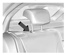
To lower the head restraint, press the button, located on the top of the seat backrest, and push the head restraint down. Try to move the head restraint after the button is released to make sure that it is locked in place.
