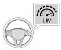
The speed limiter button is located on the steering wheel.
