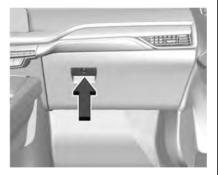
Lift the handle to open the glove box. Close until it latches. Use the vehicle key to lock or unlock. See  $Keys \Leftrightarrow 6$ .
