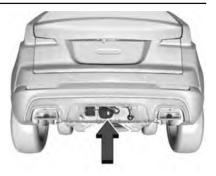
Remove the hitch cover. See "Hitch Cover" above.
