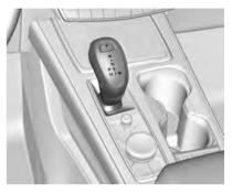
The shift pattern is displayed in the top of the gear lever. The selected gear position will illuminate red on the gear lever, while all others will be displayed in white. If the gear change is not immediate, as in very cold conditions, the indicator on the gear lever may flash until it is fully engaged.
