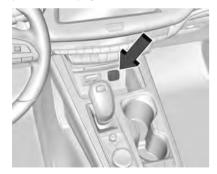
The vehicle has three accessory power sockets: one at the front of the centre console, one under the armrest, and one in the rear cargo area.
