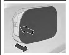
To open the fuel filler flap, push and release the rearward centre edge of the flap.
