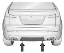
Remove the fasteners to remove the trailer hitch cover.
