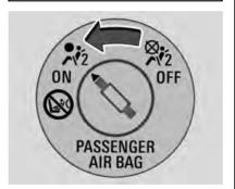
To turn the front outboard passenger airbag on again, insert the ignition key into the airbag on-off switch, push in, and move the switch to the ON position.
