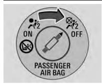
To turn off the front outboard passenger frontal airbag, insert the ignition key into the airbag on-off switch, push in, and move the switch to the OFF position.
