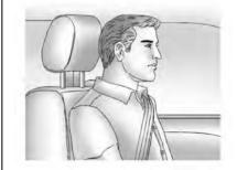
Adjust the head restraint so that the top of the restraint is at the same height as the top of the occupant's head. This position reduces the chance of a neck injury in a crash.
