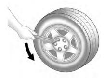
Turn the wheel wrench anticlockwise to loosen all the wheel nuts, but do not remove them yet.
