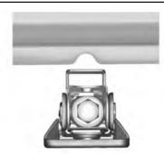
Locate the notch on the sheet metal weld flange. Place the centre of the jack lift head on the centre of the sheet metal notch.
