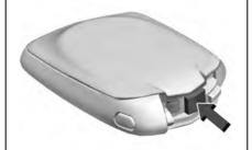
Separate the two halves of the remote key using a flat tool inserted into the bottom centre of the remote key. Do not use the key slot.
