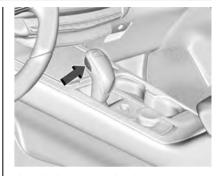
This vehicle is equipped with an electronically controlled transmission. The shift lock release button is designed to prevent inadvertent shifting out of P (Park) unless the ignition is on, the brake pedal is applied, and the shift lock release button is pressed.
