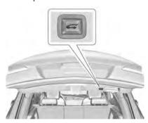
Press on the bottom of the tailgate next to the pull cup to close.
