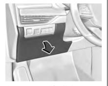
The instrument panel fuse block is on the driver side of the instrument panel, between the steering wheel and the door. To access the fuses, remove the panel, starting at the top. Once clips are disengaged, the tabs along the bottom of the door can be disengaged from the instrument panel to remove the door.
