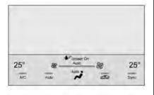
The climate control status display appears briefly when the climate controls are adjusted.
