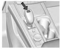
**P**: This position locks the drive wheels. Use P (Park) when starting the engine to prevent the vehicle from moving.
