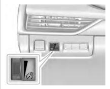
This feature adjusts the brightness of all illuminated controls. This feature is on the left side of the instrument panel.
