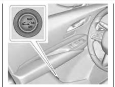
The power tailgate switch is on the driver door. The vehicle must be in P (Park).
