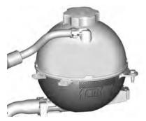
Check to see if coolant is visible in the coolant surge tank. If the coolant inside the coolant surge tank is boiling, do not do anything else until it cools down. If coolant is visible but the coolant level mark is not at
