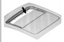
Dirt and debris may collect on the sunroof seal or in the track. This could cause an issue with sunroof operation or noise. It could also plug the water drainage system. Periodically open the sunroof and remove any obstacles or loose debris. Wipe the sunroof seal and roof sealing area using a clean cloth, mild soap, and water. Do not remove grease from the sunroof.
