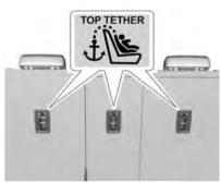
Top tether anchors are located on the back of the second row backrests and are always aligned with rear seats and identified with symbol ...
