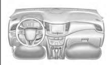
The driver knee airbag is below the steering column. The front outboard passenger knee airbag is below the glove box.
