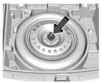
4. Turn the retainer nut anticlockwise and remove the spare tyre.
