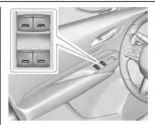
The power windows work when the ignition is on, in accessory mode, or when Retained Accessory Power (RAP) is active. See Retained Accessory Power (RAP) ⇒ 184.
