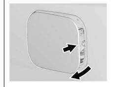
If equipped, the fuel door is locked when the vehicle doors are locked. Press on the RKE transmitter to unlock. To open the fuel filler flap. push and release the rearward centre edge of the flap.
