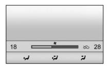
The climate control status screen appears briefly when the climate control buttons on the faceplate are adjusted. The air delivery mode can be adjusted on the climate control status screen.
