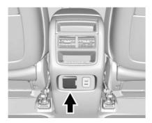
If equipped, this power outlet is on the rear of the centre floor console. It can be used to plug in electrical equipment that uses a maximum limit of 150 watts.
