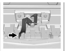
Go to the front of the vehicle to find the secondary bonnet release handle. The handle is under the front edge of the bonnet near the centre. Push the handle to the right, then raise the bonnet.
