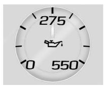
The engine oil pressure gauge shows the engine oil pressure in kPa (kilopascals) or psi (pounds per square inch) when the engine is running.
