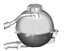
Check to see if coolant is visible in the coolant surge tank. If the coolant inside the coolant surge tank is boiling, do not do anything else until it cools down. If coolant is visible but the coolant level mark is not visible. add a 50/50 mixture of clean. drinkable water and DEX-COOL coolant at the coolant surge tank to the top rib on the middle of the tank, but be sure the cooling system is cool before this is done. See Engine Overheating \$\dip\$ 246.
