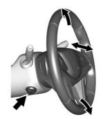
Press the control to move the tilt and telescoping steering wheel up and down or forward and rearward.
