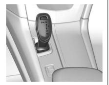
The shift pattern is displayed in the top of the gear lever. The selected gear position will illuminate red on the gear lever, while all others will be displayed in white. If the shift is not immediate, as in very cold conditions, the indicator on the gear lever may flash until it is fully engaged.
