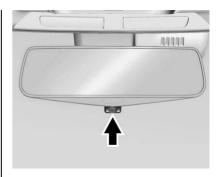
Pull the tab rearward to turn on the display. Push the tab forward to turn it off. When off, the mirror is automatic dimming. For ease of use, adjust the mirror for a clear view of the area behind the vehicle while the display is off.
