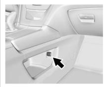
The vehicle has two accessory power sockets, one on the lower centre floor console and in the rear cargo area.
