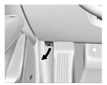
Pull the bonnet release lever with this symbol on it. It is inside the vehicle on the lower side of the instrument panel.
