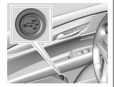
The power tailgate switch is on the driver door. The vehicle must be in P (Park).
