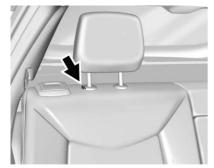
To lower the head restraint, press the button, located on the top of the seat backrest, and push the head restraint down. Try to move the head restraint after the button is released to make sure that it is locked in place.
