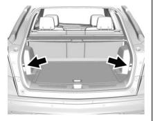
The vehicle has two cargo tie-downs in the rear compartment.
