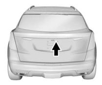
To open the tailgate, press on the power door lock switch or press on the RKE transmitter twice to unlock all doors. Press the touch pad on the underside of the tailgate handle and lift up.
