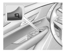
Press to power fold the mirrors. Press again to unfold.
