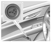
If equipped with a power tailgate, the switch is on the driver door. The vehicle must be in P (Park).
