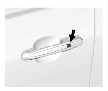
If equipped, use the Keyless Access system to lock and unlock the door. When the doors are locked and the RKE transmitter is within 1 m (3 ft) of the driver door handle, press the lock/unlock button. When unlocking from the driver door, the first press unlocks that door; press again within five seconds to unlock all passenger doors. See *Remote Keyless Entry (RKE) System Operation* ♀ 26.
