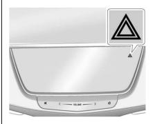
⚠: Touch ⚠ on the centre console to make the front and rear indicator lamps flash on and off. Touch again to turn the indicators off.
