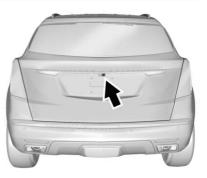
The camera that provides the RCM image is above the number plate, next to the Rear Vision Camera (RVC).
