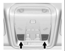
Press the lamp lenses on the front reading lamps.
