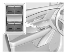
Press the switch down to lower the window. Pull the switch up to raise it. See *Power Windows*  $\Rightarrow$  47.
