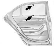
If equipped, use the handle to pull the sunshade up and attach to the holder at the top of the window. There is also a small shade for the rear corner of the window.
