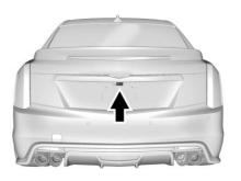
The camera that provides the Rear Camera Mirror (RCM) image is above the license plate, next to the Rear Vision Camera (RVC).
