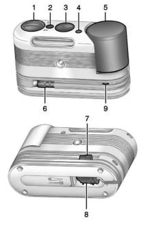
When using the tyre sealant and compressor kit during cold temperatures, warm the kit in a heated environment for five minutes. This will help to inflate the tyre faster.
