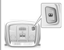
If equipped with a rear window sunshade, the switch is on the overhead console. The sunshade only operates with the ignition in ON/RUN/START.
