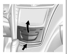
Touch the bottom of the climate control system panel until the door automatically starts to open. The storage area may contain a USB port. See the infotainment manual.
