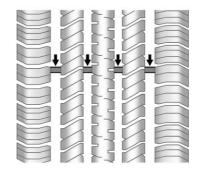
Tread wear indicators are one way to tell when it is time for new tyres. Tread wear indicators appear when the tyres have only 1.6 mm (1/16 in) or less of tread remaining. See *Tyre Inspection*  $\Rightarrow$  289 and *Tyre Rotation*  $\Rightarrow$  289.
