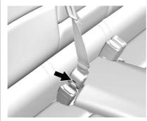
Disconnect the rear safety belt mini-latch using a key in the slot on the mini-buckle, and let the belt retract.
