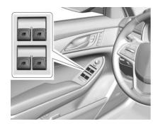
The windows work when the vehicle is in ON/RUN or ACC/ACCESSORY, or when Retained Accessory Power (RAP) is active. See *Retained Accessory Power (RAP)* ⇒ 196.
