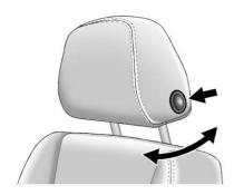
To adjust the head restraint forward and rearward, press the button located on the side facing the head restraint and move it forward or rearward until the desired locking position is reached. Try to move the head restraint after the button is released to make sure that it is locked in place.
