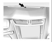
If equipped, the light sensor is on top of the instrument panel or on the windscreen near the rearview mirror. Do not cover the sensor; otherwise the headlamps will come on when they are not needed.
