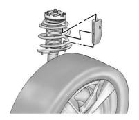
Due to low ramp angles on the V-Series only, use care when loading the vehicle onto a flatbed carrier. Front spring spacers were provided for lifting the front suspension if more clearance is necessary when towing.
