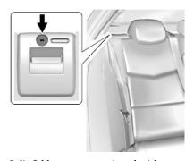
Split fold seats are equipped with a locking latch.
