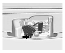
Go to the front of the vehicle to find the secondary bonnet release handle. The handle is under the front edge of the bonnet near the centre. Push the handle to the right and at the same time raise the bonnet
