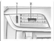
Move the slider knobs (2) to change the direction of the airflow.
