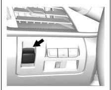
The vehicle has an Electric Parking Brake (EPB). The switch for the EPB is on the instrument panel, to the left of the steering wheel. The EPB can always be activated, even if the ignition is off. To prevent draining the battery, avoid repeated cycles of the EPB system when the engine is not running.
