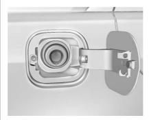
To open the fuel filler flap, push and release the rearward centre edge of the flap. The fuel door is locked when the vehicle doors are locked. Press on the RKE transmitter to unlock.
