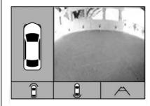
If equipped, a view of the area in front of the vehicle displays in the centre console. The view displays after shifting from R (Reverse) to a forward gear, or by pressing CAMERA in the centre stack, and when the vehicle is moving forward slower than 8 km/h (5 mph). If equipped, the front view camera also displays when the Front Parking Assist system detects an object within 30 cm (12 in).
