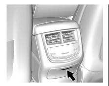
If equipped, press the top of the door to open the storage area on the rear of the centre console. If equipped, there is a power outlet inside.
