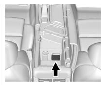
An indicator light on the outlet turns on to show it is in use. The light comes on when the ignition is in ON/RUN/START, equipment requiring less than 150 watts is plugged into the socket, and no system fault is detected.
