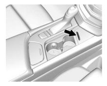
Cupholders in the front centre console have a power retractable cover. Push the handle forward to express open. Pull the handle rearward to express close.
