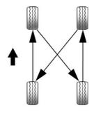
Use this rotation pattern when rotating tyres of the same size installed on all four wheel positions.
