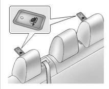
Top-tether fastening eyes are marked with so for a child seat.
