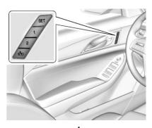
The SET, 1, 2, and (E) (Exit) buttons on the driver door are used to manually store and recall memory settings for the driver seat, outside mirrors, power tilt and telescoping steering column (if equipped).
