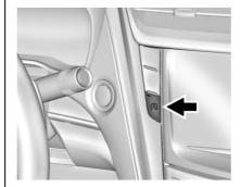
The automatic engine stop/start function can be disabled using the switch to the left of the infotainment display. The indicator on the switch will illuminate when the system is operational.
