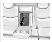
The vehicle has a rear seat pass-through door in the centre of the rear backrest. Fold down the center armrest and pull the lever all the way down to release the door.
