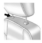
To lower the head restraint, press the button, located on the top of the seat backrest, and push the head restraint down. Try to move the head restraint after the button is released to make sure that it is locked in place.
