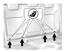
ISOFIX mounting brackets are marked by on the seat back.
