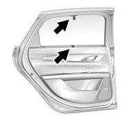
If equipped, use the handle to pull the sunshade up and attach to the holder at the top of the window.
