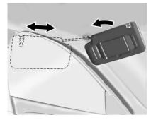
Pull the sun visor down to block glare. Detach the sun visor from the centre mount to pivot to the side window, or to extend along the rod.
