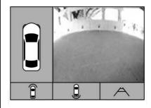
If equipped, a view of the area in front of the vehicle displays in the infotainment display. The view displays after shifting from R (Reverse) to a forward gear, or by pressing CAMERA in the centre stack, and when the vehicle is moving forward slower than 8 km/h (5 mph). If equipped, the front view camera also displays when the Front Parking Assist system detects an object within 30 cm (12 in).
