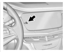
The automatic engine stop/start function can be disabled by touching  $\widehat{A}$  on the infotainment display. The indicator next to the switch will come on when the system is active.
