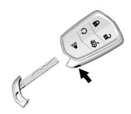
This key, inside the Remote Keyless Entry (RKE) transmitter, is used for the driver door.
