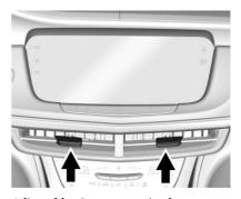
Adjustable air vents are in the centre and on the sides of the instrument panel, on the rear of the centre console storage, and in the headlining over the rear seats, if equipped.
