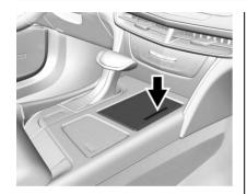
There are cupholders in the centre console. Push and release on the passenger side of the cover to access the cupholders.
