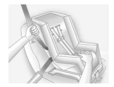
To tighten the belt, push down on the child restraint, pull the shoulder portion of the belt to tighten the lap portion of the belt, and feed the shoulder belt. back into the retractor. When installing a forward-facing child restraint, it may be helpful to use your knee to push down on the child restraint as you tighten the belt.
