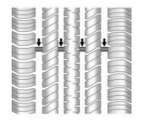
Tread wear indicators are one way to tell when it is time for new tyres. Tread wear indicators appear when the tyres have only 1.6 mm (1/16 in) or less of tread remaining. See *Tyre Inspection*  $\Rightarrow$  281 and *Tyre Rotation*  $\Rightarrow$  281.
