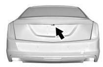
The camera that provides the Rear Camera Mirror (RCM) image is above the license plate, next to the Rear Vision Camera (RVC).
