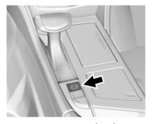
Automatic Vehicle Hold (AVH) can be turned on by pressing AUTO HOLD with the driver seat belt fastened, the driver door closed, and the engine running. The AVH indicator will come on.
