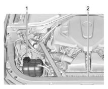
Engine Coolant Surge Tank and Pressure Cap 2. Engine Cooling Fan (Out of View)
