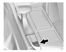
Press and release MODE on the centre console to activate the mode menu in the instrument cluster. The first press of the button will show the current mode. Subsequent presses will scroll through the available modes. Select a new setting whenever driving conditions change. The following modes are available:
