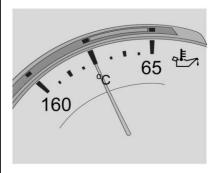
This gauge shows the engine oil temperature.
