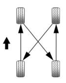
Use this rotation pattern when rotating tyres of the same size installed on all four wheel positions.
