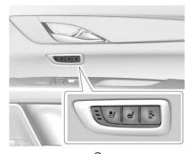
If equipped, press to return the seat to the full rearward and full front of seat tilt down position. The seat will also move to this position when the rear door is opened.
