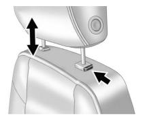
Pull the head restraint up to raise it. Try to move the head restraint to make sure that it is locked in place.
