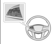
(S): Press to turn the system on and off. A white indicator appears in the instrument cluster when turned on.
