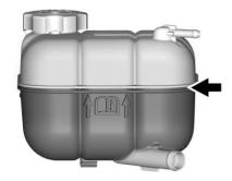
Check to see if coolant is visible in the coolant surge tank. If the coolant inside the coolant surge tank is boiling, do not do anything else until it cools down. If coolant is visible but the coolant level mark is not visible. add a 50/50 mixture of clean. drinkable water and DEX-COOL coolant at the coolant surge tank to
