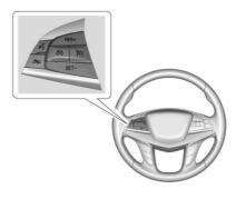
(5): Press to turn the system on and off. A white indicator appears in the instrument cluster when cruise is turned on.
