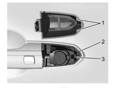
Insert the tabs (1) on the rear of the cap into the space between the seal (2) and the metal base (3).
