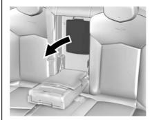
Some vehicles have a rear seat pass-through door in the centre of the rear seatback. Fold down the centre armrest and pull the latch to open the door.
