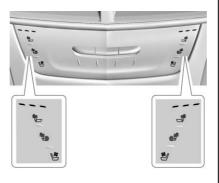
If equipped, the buttons are near the climate controls on the centre stack. To operate, the ignition must be in ON/RUN.
