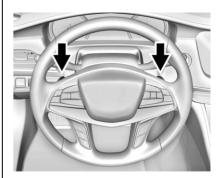
Vehicles with Tap Shift have controls on the back of the steering wheel to manually shift the automatic transmission. To enter Permanent Tap Shift Mode:
