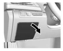
The storage compartment has a press to open latch. To access the fuses, open the compartment by pressing and releasing near the top centre square.
