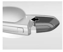
3. Move the cap inward and press to snap the cap in place.
