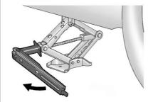
Raise the vehicle by turning the jack handle clockwise. Raise the vehicle far enough off the ground so there is enough room for the road tyre to clear the ground.
