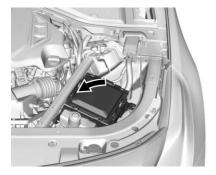
Lift the fuse block cover to access the fuses.
