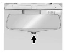
Pull the tab rearward to turn on the display. Push the tab forward to turn it off. When off, the mirror is automatic dimming. Adjust the mirror for a clear view of the area behind the vehicle while the display is off.
