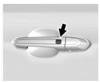
Press the lock/unlock button when the RKE transmitter is within 1 m (3 ft) of the driver door handle. When unlocking from the driver door, the first press unlocks that door; press again within five seconds to unlock all passenger doors. See *Remote Keyless Entry (RKE) System Operation* ⇒ 28.
