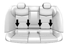
ISOFIX mounting brackets are marked by on the seat back.
