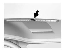
The solar sensor, on top of the instrument panel near the windscreen, monitors the solar heat.
