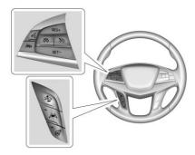
The Collision Alert control is on the steering wheel. Press to set the FCA timing to Far, Medium, or Near, or on some vehicles, Off. The first button press shows the current setting on the DIC. Additional button presses will change this setting. The chosen setting will remain until it is changed and will affect the timing of both the Collision Alert and the Tailgating Alert features. The timing of both alerts will vary based on vehicle speed.
