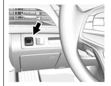
The vehicle has an Electric Parking Brake (EPB). The EPB can always be activated, even if the ignition is off. To prevent draining the battery, avoid repeated cycles of the EPB system when the engine is not running.
