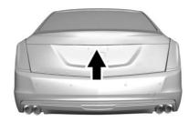
Press the touch pad on the rear of the boot above the number plate when all doors are unlocked.
