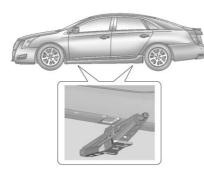
8. Position the jack lift head at the jack location nearest the flat tyre within the depression of the jack
