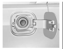
To open the fuel filler flap, push and release the rearward centre edge of the flap. The fuel door is locked when the vehicle doors are locked. Press on the RKE transmitter to unlock.
