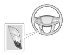
**3**: If equipped with a heated steering wheel, press to turn on or off. An indicator next to the button is lit when the feature is turned on
