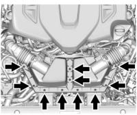
Remove the 10 screws on top of the engine air cleaner/filter cover to gain access to both air cleaner/filters.
