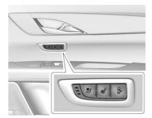
If equipped, the buttons are on the rear passenger doors.
