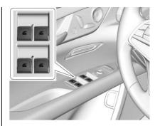
The windows work when the vehicle is in ON/RUN, ACC/ACCESSORY, or Retained Accessory Power (RAP). See *Retained Accessory Power* (RAP)  $\Rightarrow$  198.
