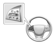
(S): Press to turn the system on or off. A white cruise control indicator comes on.
