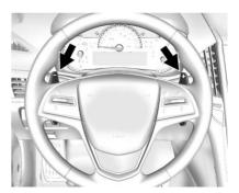
If equipped, the tap shift controls are on the back of the steering wheel.
