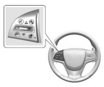
The Collision Alert control is on the steering wheel. Press to set the FCA timing to Far, Medium, Near, or on some vehicles, Off. The first button press shows the current setting on the DIC. Additional button presses will change this setting. The chosen setting will remain until it is changed and will affect the timing of both the Collision Alert and the Tailgating Alert features. The timing of both
