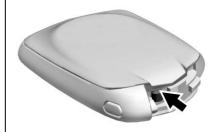
Separate the two halves of the transmitter using a flat tool inserted into the bottom centre of the transmitter. Do not use the key slot.
