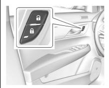
**:** Press to lock the doors. The indicator light in the switch will illuminate when activated.
