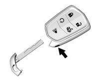
Press the button on the side of the transmitter near the bottom and pull the key out.
