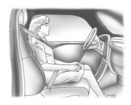
If a person of adult size is sitting in the front outboard passenger seat, but the off indicator is lit, it could be because that person is not sitting properly in the seat. Use the following steps to allow the system to detect that person and enable the front outboard passenger frontal airbag and knee airbag:
