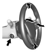
If equipped, the control is on the left side of the steering column.
