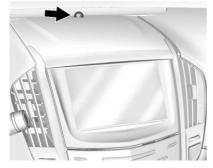
There is a light sensor on top of the instrument panel. Do not cover the sensor; otherwise the headlamps will come on when they are not needed.
