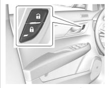
From the inside, press  $\bigcirc$  or  $\bigcirc$ . The indicator light in the switch will illuminate when locked. See *Power Door Locks*  $\Rightarrow$  35.
