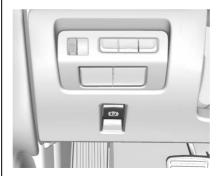
If equipped with an Electric Parking Brake (EPB), the switch is on the left side of the instrument panel. The EPB can always be activated, even if the ignition is off. To prevent draining the battery, avoid repeated cycles of the EPB when the engine is not running.
