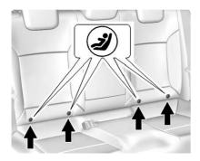
ISOFIX mounting brackets are marked by **2** on the seat back.
