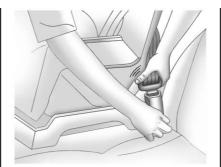
Push the latch plate into the buckle until it clicks. If the latch plate will not go fully into the buckle, check if the correct buckle is being used.
