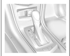
**P**: This position locks the rear wheels. Use this position when starting the engine because the vehicle cannot move easily.
