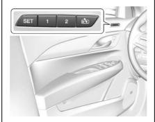
The 1, 2, SET, and (Ext) buttons on the driver door are used to manually save and recall memory settings for the driver seat, outside mirrors, and power tilt and telescoping steering column (if equipped).
