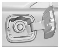
The coupé vehicle has a capless refuelling system and does not have a fuel cap. The filling nozzle must be fully inserted and latched prior to starting fuel flow.
