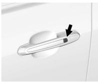
If equipped, use the Keyless Access system to lock and unlock the door. When the doors are locked and the RKE transmitter is within 1 m (3 ft) of the driver door handle, press the lock/ unlock button. When unlocking from the driver door, the first press unlocks that door; press again within five seconds to unlock all passenger doors. See *Remote Keyless Entry (RKE) System Operation* ♀ 27.
