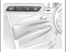
If equipped, the 1, 2, SET, and (Exit) buttons on the driver door are used to manually store and recall memory settings for the driver seat, outside mirrors, and power tilt and telescoping steering column (if equipped).
