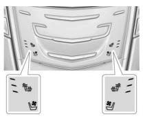
If equipped, the buttons are near the climate controls on the centre stack. To operate, the ignition must be on.
